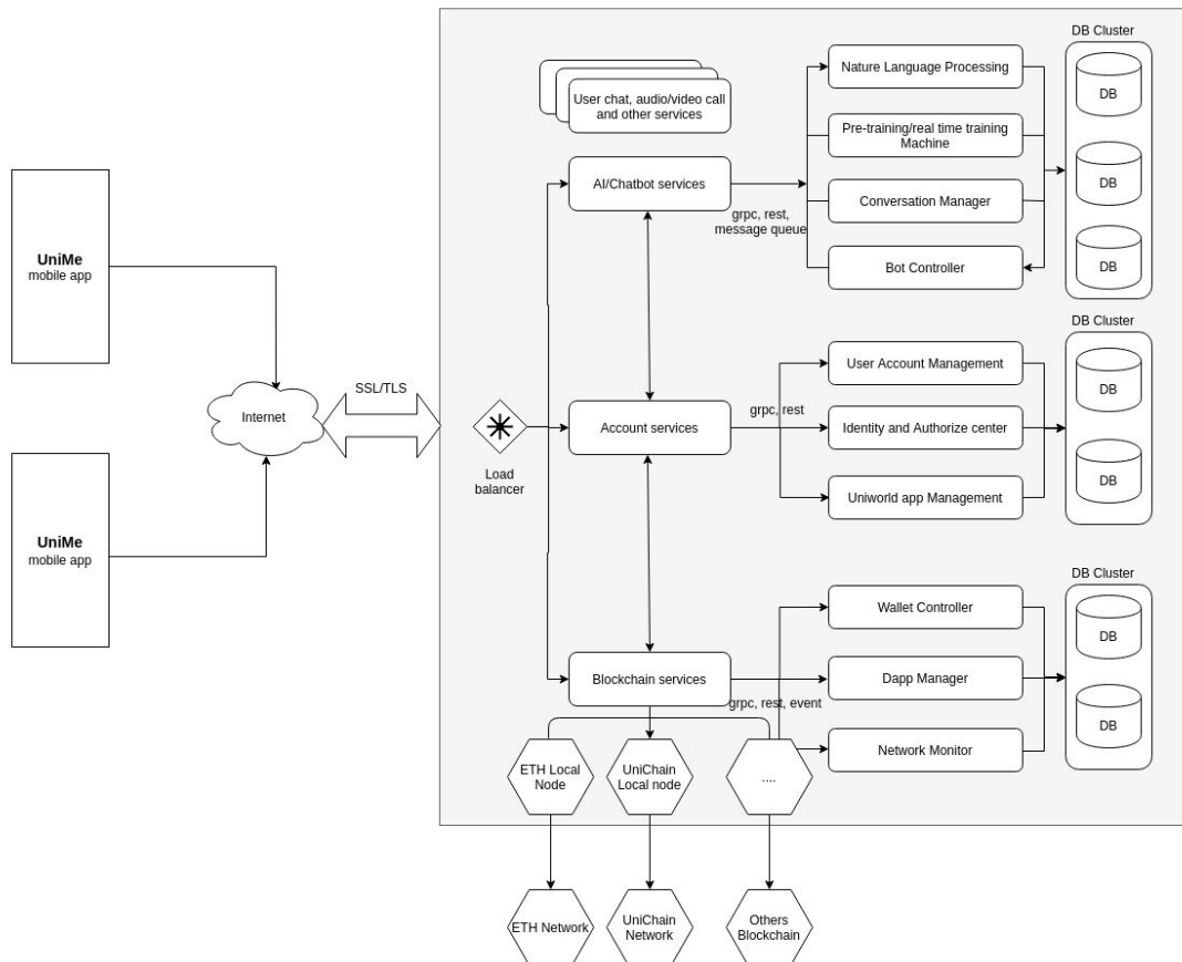
Fig. 1. UniMe application high level architecture illustrated.
